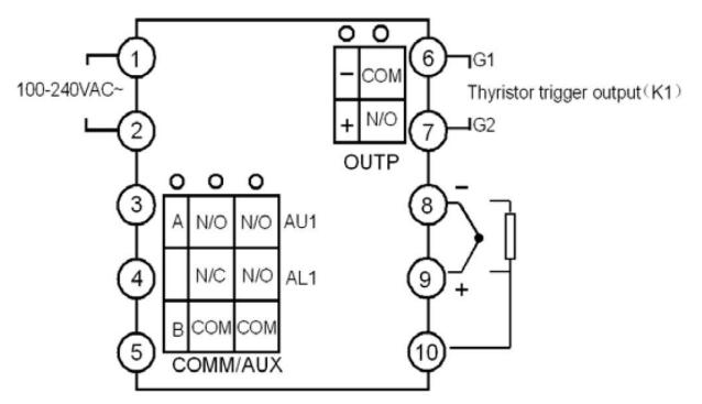
Wiring graph of instruments with D5 dimension as below:
