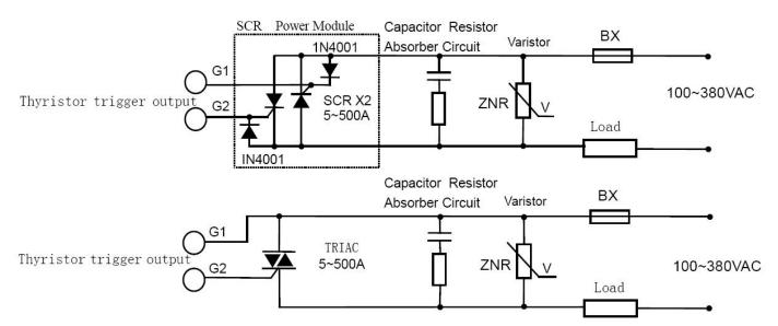
Note 1: According to the voltage and current of load, choose a suitable varistor to protect the thyristor.
