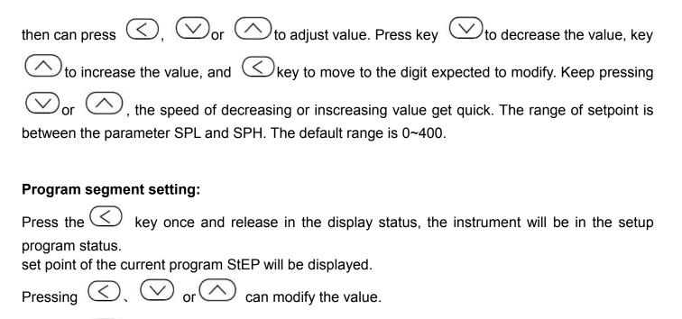
Pressing  $\bigcirc$  can go to next parameter. The program parameters will be displayed in the sequence
