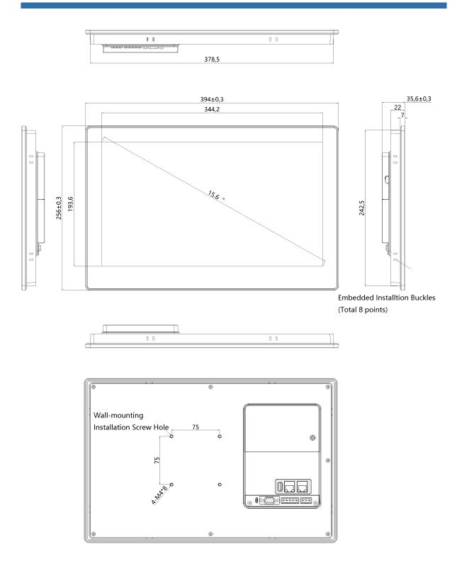
${\small Embedded\ Installtion\ Hole\ Dimension\ :\ 380mm^*245mm}$
