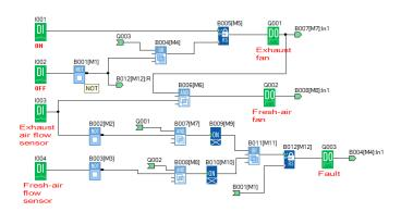
You can invert output Q3 to use output messages at Q4. Relay Q4 only drops out if main power is lost or if there is a fault in the system. The output can then be used for a remote message.
