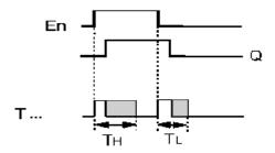
With the 0 to 1 transition at input En, a random time (on delay time) between 0 s and  $T_{\rm H}$  is set and triggered. If the status at input En is 1 at least for the duration of the On delay, the output is set to 1 when this On delay time has expired.
