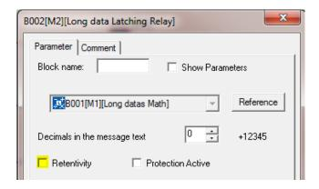
When the Input I001 is High, block B002 stores the current value of block B001.
