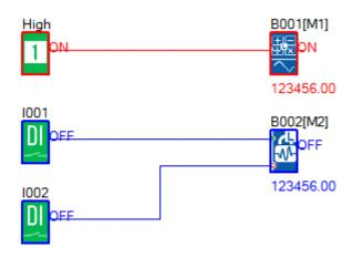
A High state at the Reset pin, resets the value to 0.
