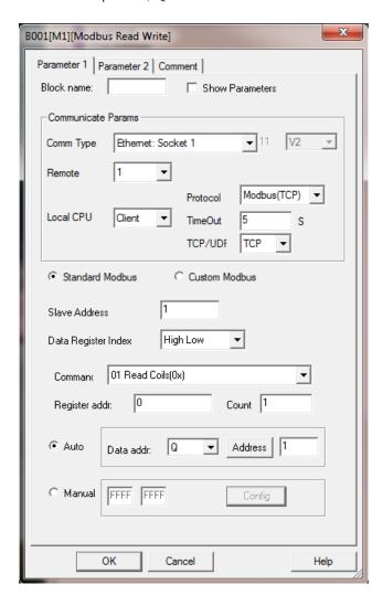
Remote 1 is the channel that belongs to the Slave and its IP address (192.168.0.227) and port number (5001) is configured using Tools  $\rightarrow$  Transfer  $\rightarrow$  Web Server Config:
