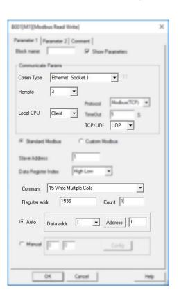
B003 is used to transfer I1 status to the F1 of slave3 by UDP connection.
