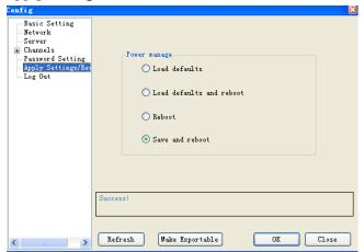
To enable any changes to be permanently saved to the xLogic Ethernet CPU you must select the Save and reboot option and press the OK button.
