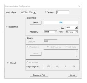
c. Click connect to PLC button to establish communications between PC and PLC.
