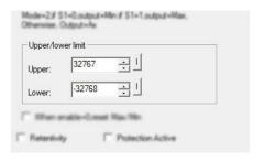
In the dialogue box of Max/Min block, there is an upper/lower limit setting, when the block output the AQ value is less than the lower value, the AQ shall be equal to the Lower value; While the block output the AQ value is more than the upper value, the AQ shall be equal to the upper value.
