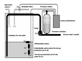
The rainwater is collected in the container and then pumped to service water pipework via the pump M1. The system allows the tank to also be filled from the drinking water supply when there is not enough rain water.
