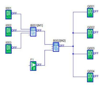
2. Clicking on a Digital Input block with the mouse will change the state of the input. The state displays "ON" and "OFF" on the output side of the block, so you can observe the state of input or output.
