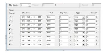
If we set Max Clients to 0, then the CPU will only act as a TCP Client, and 8 TCP servers can be connected at the same time.
