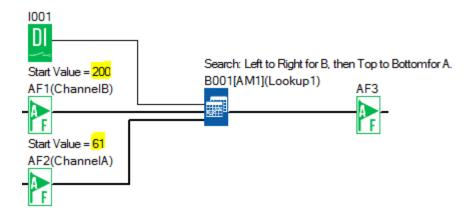
In the above program, AF1 has a Start Value of 200 (Channel B) and AF2 has a Start Value of 61 (Channel A). When the digital input I001 is On (High), the analogue table will look-up the values, B followed by A, and output the table value, which will be stored in AF3.
