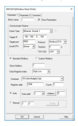
B002 is used to transfer the I1 status to the F1 of slave2 (slave2 IP 192.168.0.102, UDP port is 8002)
