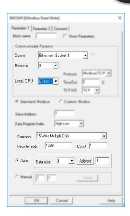
B003 is used to write I1 status to F1 of slave1, the Remote 3 is the target3 in the network parameter settings.
