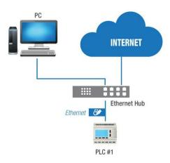
The Ethernet CPU default IP address is 192.168.0.250 and the network mask is 255.255.255.0.
