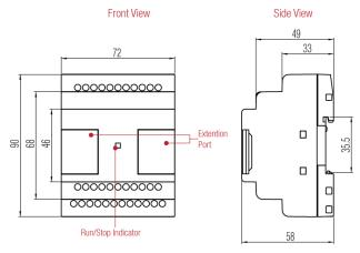
**Figure 11 PR-E Expansion Modules**
