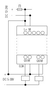
**Figure 24 Transistor Digital Output**
