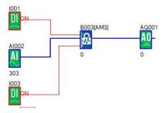
1. Start value – You can set a start value for the data latch relay block, which can be a fixed value or use the value from an existing programmed block by using the 'Reference' button.
