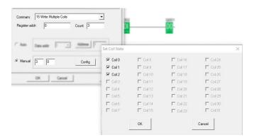
The above configuration is to force Q1, Q2, Q3 of Slave No.1 ON. Coil 0 "means pre-set the BIT 1 and "means pre-set the BIT 0 "Coil 0" is corresponding to the start address, Here it is Q1.
