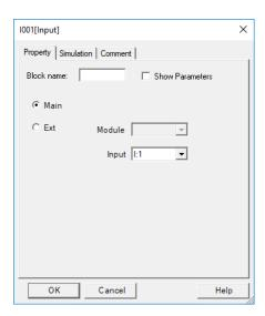
Figure 40 - Digital Input Block Configuration
