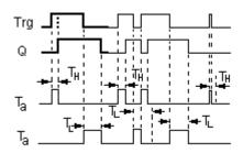
The time  $T_{\text{H}}$  is triggered with a 0 to 1 transition at input Trg.
