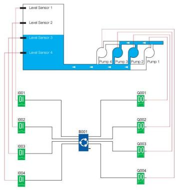
The "number of outputs controlled" parameter is fixed at 4.
