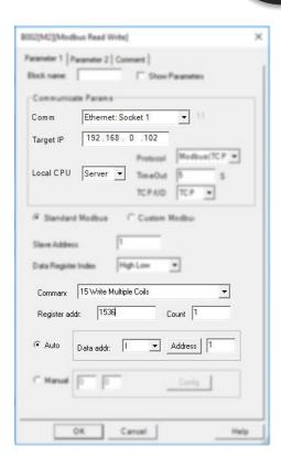
If B002 is enabled, the I1 status of master will transferred to the F1 (Modbus address is 0x1536) slave2 (IP:192.168.0.102).
