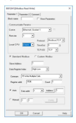
B001 is used to write I1 status to F1 of slave1, the Remote 1 is the target1 in the network parameter settings.
