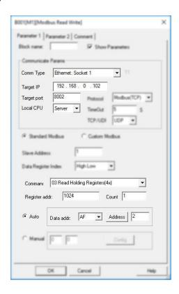
B005 is used to read the AI1 value from slave2, then save it into AF2 of master (slave1 IP 192.168.0.102, UDP port is 8002)
