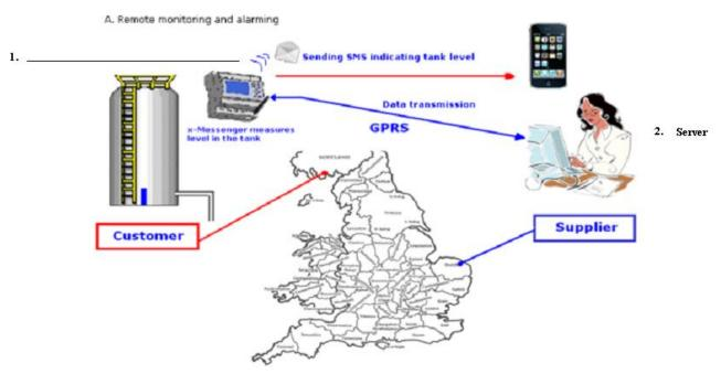
When EXM CPU is acting as Server with a FIXED IP address and office Client software requesting information such as level, temperature, digital states, etc.
