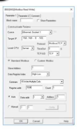
If B003 is enabled, the I1 status of master will transferred to the F1(Modbus address is 0x1536) slave3 (IP:192.168.0.103).
