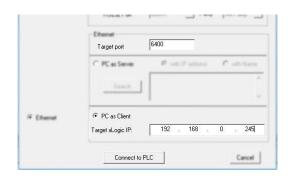
After the connection is established, you can download/upload the program and monitor the program just like using the USB cable connection.
