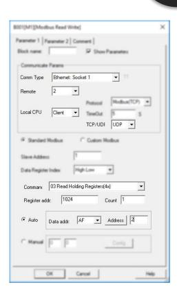
B005 is used to read AI1 value from slave2 and save the value into AF2 by UDP connection.
