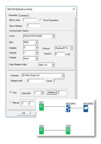
I1 of the master is used to control the communication. If I1 is high and the communication is established successfully, one alarm message (text message block) will be displayed on the LCD. Then Q1 of slave No.1 will be controlled by I2 of the master. If I2 is high, Q1 of slave No.1 would be ON and if I2 is low, Q1 of the slave would be OFF.
