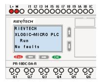
After pressing ESC key, xLogic switches to function page and the function menu will be shown as below.
