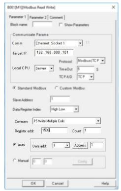
If B001 is enabled, the I1 status of master will transferred to the F1 (Modbus address is 0x1536) slave1 (IP:192.168.0.101).
