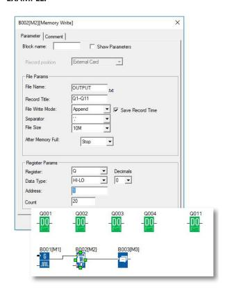
Please refer the property dialogue box of B002, it can record the output status. The start address is from 1 and it must record the 20 outputs with continuous addresses.
