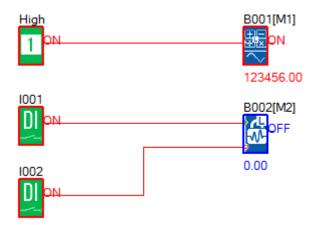
If the Reset pin is set to OFF, the value retained is still 0 because the Set pin only triggers a storing of the referenced value with a Low to High transition.
