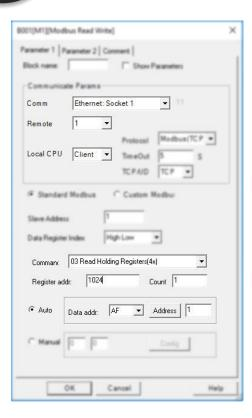
B004 is used to read AI1 value of slave1 then save into AF1, the Remote 1 is the target1 in the network parameter settings.
