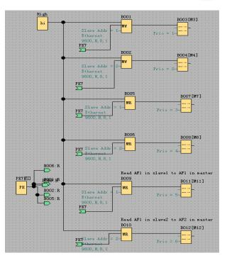
B001: Transfer the I1--IA status of the Master to the Q1-QA of the Slave1. Settings are as follows:
