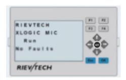
Press "Set" = Press OK key for 3 seconds then the parameters in the text message block can be modified in the usual way using the cursor keys.
