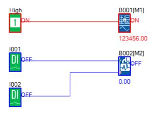
The Long Data Latching Relay block (B002) is configured to reference B001. Note that is Retentivity is checked, then the value in memory will be reserved on power cycle of the PLC. If Protection Active is checked, then user will be unable to change the blocks value via the PLC LCD.
