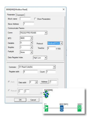
If the count was set to 4, then Q1, Q2, Q3, Q4 of xLogic (Slave No.1) would be read and saved flags F1 to F4 of the Master CPU.
