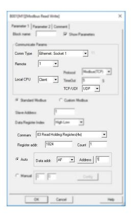
B004 is used to read AI1 value from slave1 and save the value into AF1 by UDP connection.
