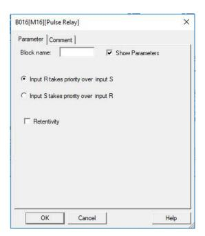
Either the input R takes priority over input S (i.e. the signal at input S has no effect as long as R = 1), or the input S takes priority over input R (i.e. the signal at input R has no effect as long as S = 1), depending on your configuration.
