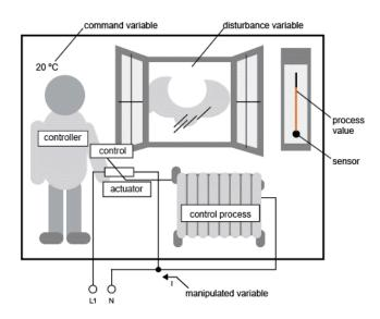
The control device is formed from the actuator and the control.
