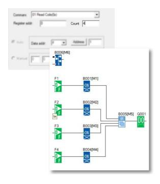
F is bit type flag. It can be used to receive bit data from a slave device.
