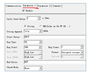
Transmit the characters "ABCD" and the value in block VB0 and "EOF" (End Data) and a Carriage Return with Line Feed via COM 0.
