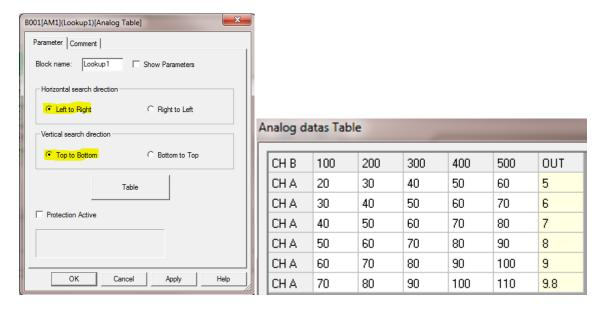
When DI1 = On, the table will be searched for the value of Channel B (200) from Left to Right and then for the value of Channel A (61) from Top to Bottom. In this example the value passed to AF3 will be 8 \* 100 = 800.
