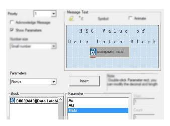
There is a Modbus address for the HEG, so you can also change the HEG value by a Modbus Master (Touchscreen etc.). You can find the address in the Modbus RTU User Manual or written in next to the block in your program.
