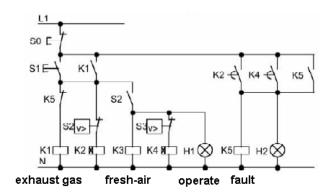
The fans are monitored by means of flow sensors. If no airflow is registered after a short delay time has expired, the system is switched off and an error message is generated, which can be acknowledged by pressing an Off button.
