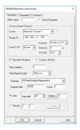
If B004 is enabled, the master will read the AI1 value (Modbus address 4x1024) of slave1 and save into local AF1.
