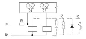
Figure 23 Relay Digital Output
