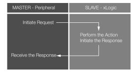
However, the "Modbus Read" or "Modbus Write" (see next chapter) function blocks should be used if xLogic shall be required to play a role of master to communicate with other slave devices. As the following figure shows:
