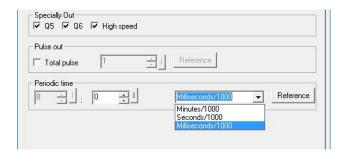
If the special output is selected in the property dialogue box of PWM block, then the unit of "periodic time" will be changed from s:1/100s to s:1/1000s, so if you input 3 (1/1000s), then its frequency will be 1000/3 Hz.
