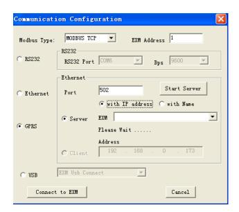
Ensure the port number is set to 5002 if this was used as in our example and press the 'Start Server' button to create a GPRS connection between the PC and the EXM CPU. After connection is established, you are able to upload/download programs and remotely monitor the CPU from anywhere in the world!!!
