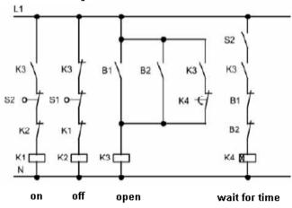
As long as the detector B1 or B2 detects someone approaching, the switch, K3 will be on and open the door.
