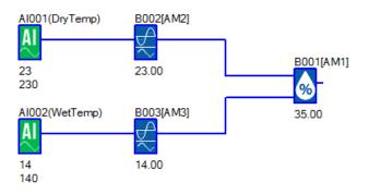
With a measured Dry temperature of 23  $^{\circ}\text{C}$  and Wet temperature of 14  $^{\circ}\text{C}$  at 101.3 kPa gives a Relative Humidity of 35%.
