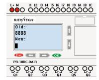
Input nothing under the "New" and press OK to clear the password.
