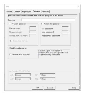
Program password and parameter password can be set here. You can also directly set the parameter password by the HMI on the CPU if fitted using "Set.."->" Password"->"Set password".
