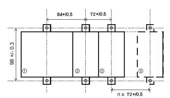
Figure 14 PR-18 & Expansions Wall Mounts
