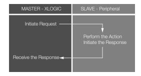
When you put the "Modbus read" or "Modbus Write" function block in your program the xLogic CPU will behave as a Modbus RTU Master.
