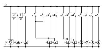
The lighting arrays can be operated by a pulse relay controlled by a button beside the door. This can be replaced by means of a timer and photosensor. The pulse relay may shorten the pulse width of the "off command".
