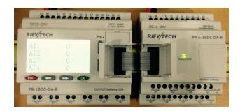
Figure 13 Connection the CPU with expansion
