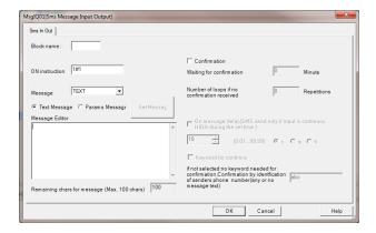
This block can be used when you require a SMS message to be sent on an event AND you require an acknowledgement from the receiver.
