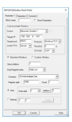
B001 is used to transfer the I1 status to the F1 of slave1 (slave1 IP 192.168.0.101, UDP port is 8001)
