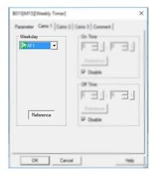
In order to set the weekly timer parameters via MODBUS, they can be assigned to an Analogue flag, AF, which would hold a value to represent the bits for each day of the week.
