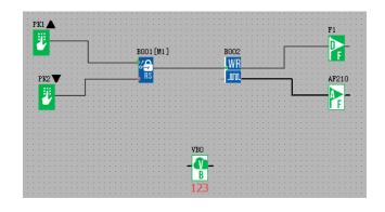
When Up arrow on CPU is pressed, transmitting begins and is stopped by pressing Down arrow on CPU.
