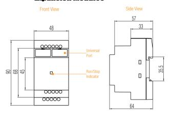
Figure 4 PR-6 Series CPU and EXM-E Dimensions
