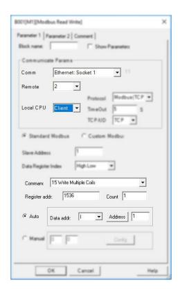
B002 is used to write I1 status to F1 of slave1, the Remote 2 is the target2 in the network parameter settings.
