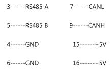
Communication between CPU and expansion module will use pins 4, 7, 9 and 15.
