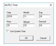
If you check the tick box "Use System Time" then the PC time and date will automatically be entered, otherwise adjust enter parameter as required and when done press the "Ok" button.
