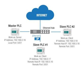
First, you must configure each xLogic Ethernet CPU with its own unique settings using the Device Manager software.
