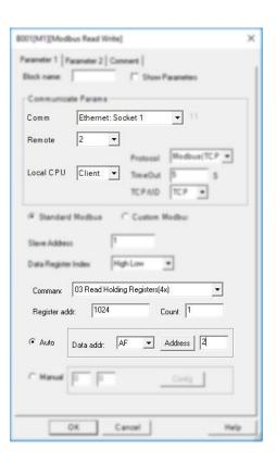
B005 is used to read AI1 value of slave2 then save into AF2, the Remote 2 is the target2 in the network parameter settings.
