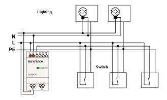
The wiring of a lighting system with xLogic is the same as standard corridor or stairway lighting systems. Only the automatic lighting timer/pulse relay is replaced.
