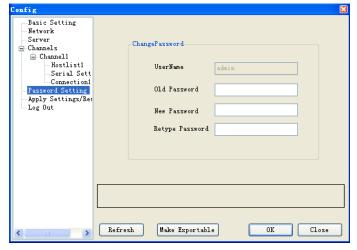
A password must be provided to communicate via the xLogic CPU Ethernet port and can be changed here. The default password is admin. The password must contain at least one character.
