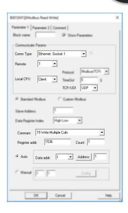
B001 is used to transfer I1 status to the F1 of slave1 by UDP connection.
