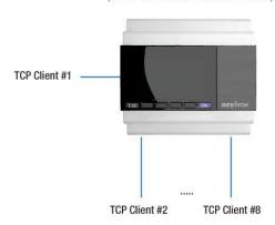
All the 8 Servers can be connected, and the data transmission can be processed separately.
