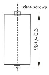
Figure 12 PR-6 Wall Mounting
