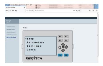
You can change any data using the web page that can be changed via the LCD and physical buttons on the screen.
