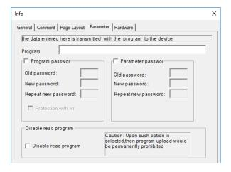
There are 2 password settings which can be applied to the program, one is the program password and the other is the parameter password.
