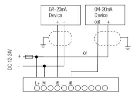
Figure 21 Analogue Current Inputs
