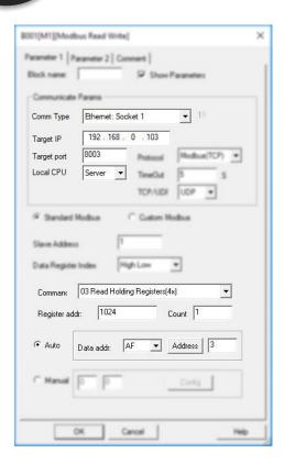
B006 is used to read the AI1 value from slave3, then save it into AF3 of master (slave1 IP 192.168.0.103, UDP port is 8003)
