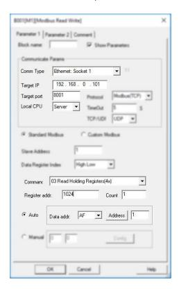
B004 is used to read the AI1 value from slave1, then save it into AF1 of master (slave1 IP 192.168.0.101, UDP port is 8001)
