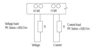
Figure 25 Analogue 0-10V and 0-20mA Output
